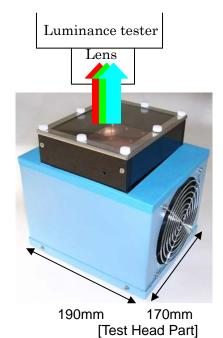
This Compact Temperature Chamber RK-10207P allows the user to make the target light emitting element hot or cool up to the specified temperature and keep the temperature. It is best suitable to test light emitting display panel, test element such as LCD, OLED and LED, and large scale IC module and others.
