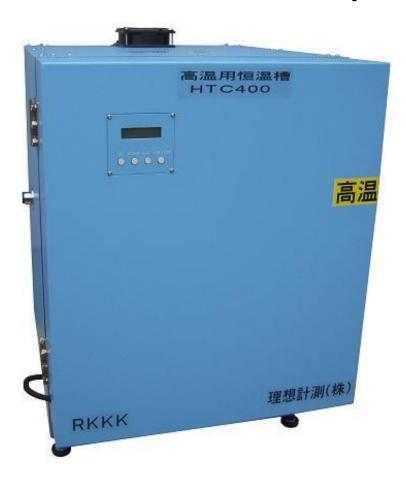
RT to +400°C T-range SiC Power Semiconductor High Temp Storage test, High Temp Bias test Inner size: 30x30x30 cm<sup>3</sup> Direct Heat Transfer method:  $+/- 1.0^{\circ}C (at 400^{\circ}C)$ Small outside size: 60Wx69Dx70Hcm<sup>3</sup>
