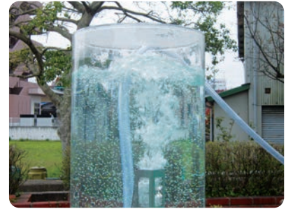
③ Sludge stirred in a tube churns in a spiral and circulates in the tank for purification.
