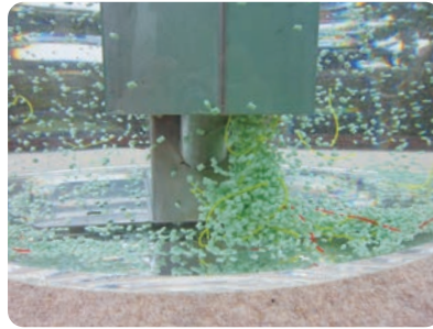
② Sludge drawn into a tube rises while colliding against and stirring with air and turning.
