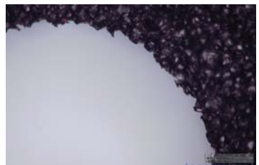
Cut edge with other company's hole punch
