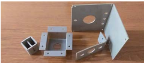
PEEK bending samples
