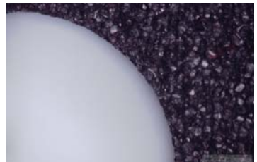
Cut edge with sharpened blade (enlarged)
